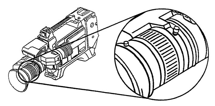
FIGURE 1-3. MANUAL FOCUS CONTROL RING
