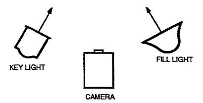
FIGURE 2-3. BASIC THREE-POINT LIGHTING SCHEME
