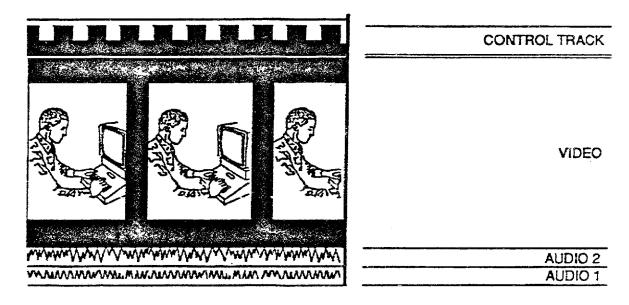
FIGURE 4-2. TRACK LOCATION, 3/4" VIDEOTAPE
